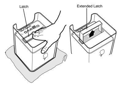
7 Gently pull the core from the computer enclosure and place the core on a soft cloth. (Figure 3)
